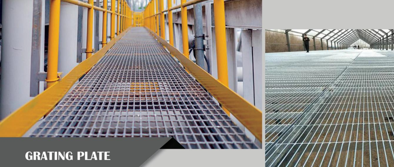
Riveted Grating Exceptionally durable grating manufactured by riveting bearing bars and bent connecting bars at their contact points.
